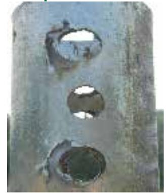
Competitor pipe piles are held together and rotated by the bolts alone. Torsion results in elongating the hole and reducing pipe strength and stability.
