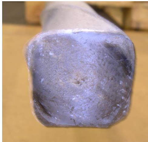
View of shaft at break point
