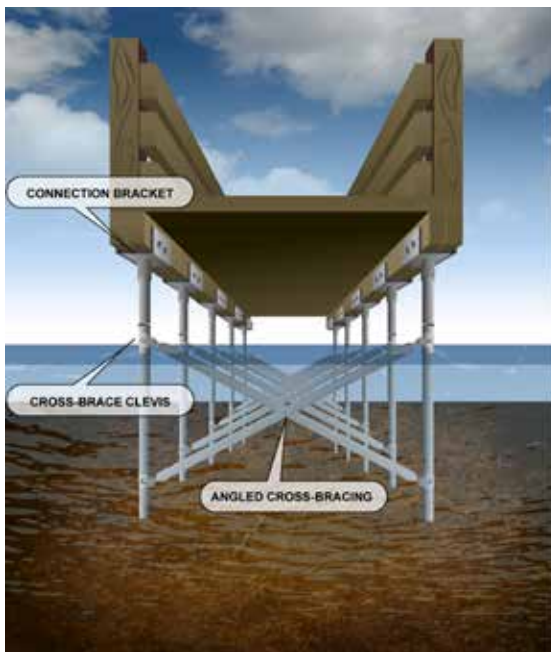
Example of cross bracing for lateral support.
